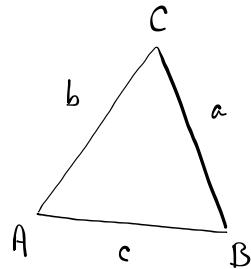
$$\frac{a}{\sin A} = \frac{b}{\sin B} = \frac{c}{\sin C} \quad (\text{finding a side})$$
